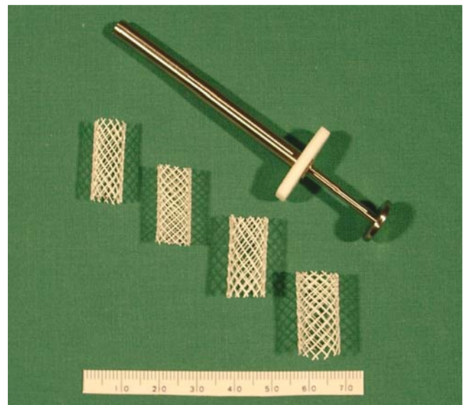
Figure 1 The braided, self-reinforced, gamma-sterilized PLA–BaSO 4 BDBSs (length 20 mm, outer diameters 6, 7, 8, and 9 mm when fully expanded) used in the HJ anastomosis in group I animals and the custom-made applicator for introducing the stent.
